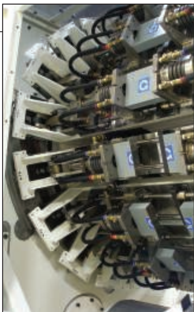
FIGURE 3. A configurable rotary-wheel extrusion blow molder allows for high outputs of a range of bottle sizes used in beverage, dairy and household products on a single platform
