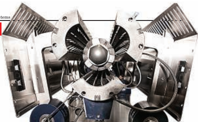
FIGURE 1. The TriVolution offers twelve pin-flight intermeshing zones in the cross section, versus two for a typical twin-screw extruder or three for a typical continuous kneader
