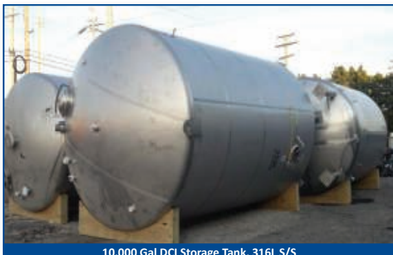
10,000 Gal DCI Storage Tank, 316L S/S
